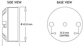
Fixing holes 2 x Ø5.5 mm, Centre hole Ø4.5 mm
